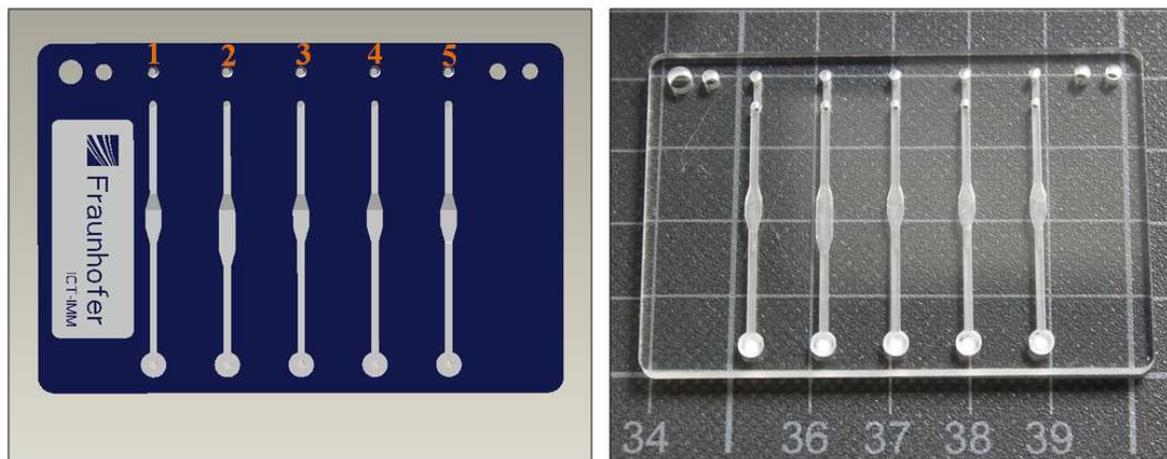
Figure 6: Preliminary design of a reservoir chip to pre-store reagents. 1) ion low calibration, 2) ion high calibration, 3) isotonic solution; 0.9% NaCl 4) isotonic solution, and 5) bilirubin reference solution.
