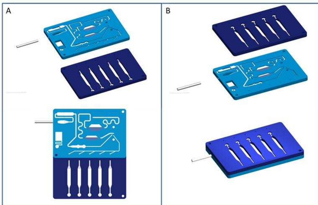
Figure 7: Possibilities to join the reservoir chip (dark blue) and the microfluidic cartridge (light blue) to the master chip. Design A is favoured.
