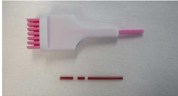
Figure 2: Disposable device for finger pricking and an incompletely filled capillary
