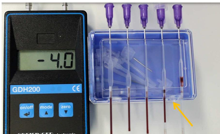
Figure 3: Pressure difference to transfer the blood from the filled capillary into the cartridge (arrow).
