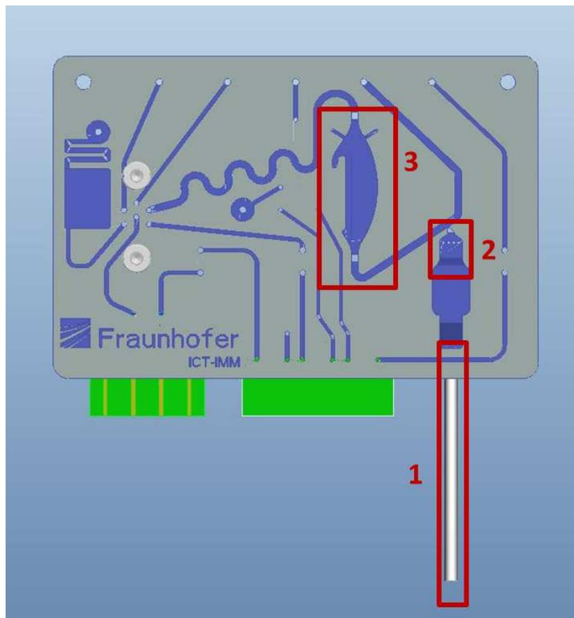
Figure 1: Pre-final microfluidic cartridge with microfluidic modules highlighted in red.
