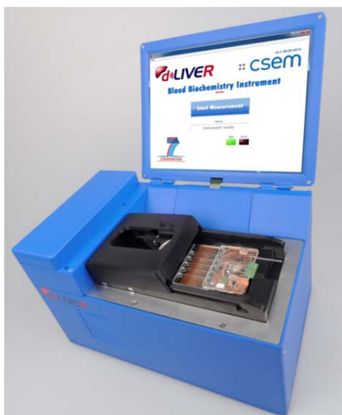
Figure 4: Blood Biochemistry Instrument with BBC in place. The action of closing the cover over the BBC automatically assembled both of the cartridge components.
